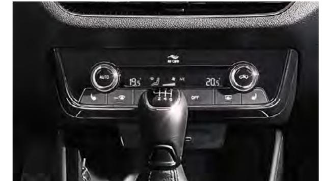
DUAL ZONE AIR CONDITIONING WITH CLIMATRONIC ELECTRONIC CONTROL
